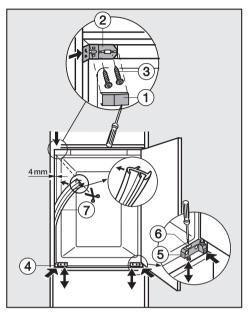
■ Plug the gap between the appliance and the furniture wall on the door opening side with sealing strip ⑦. Press the sealing strip into the gap starting at the bottom, and cut to length so that it fits snugly to the
